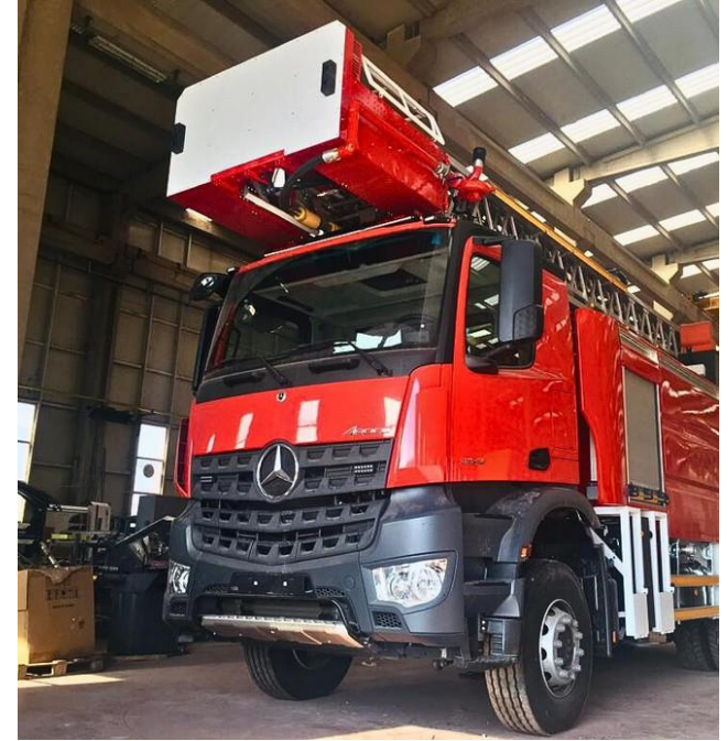
Mercedes Benz Arocs 6x4 Truck; superstructure 28 meters ladder fire extinguishing truck with 4 tons of water + 2 tons of foam tank capacity with folding type basket
