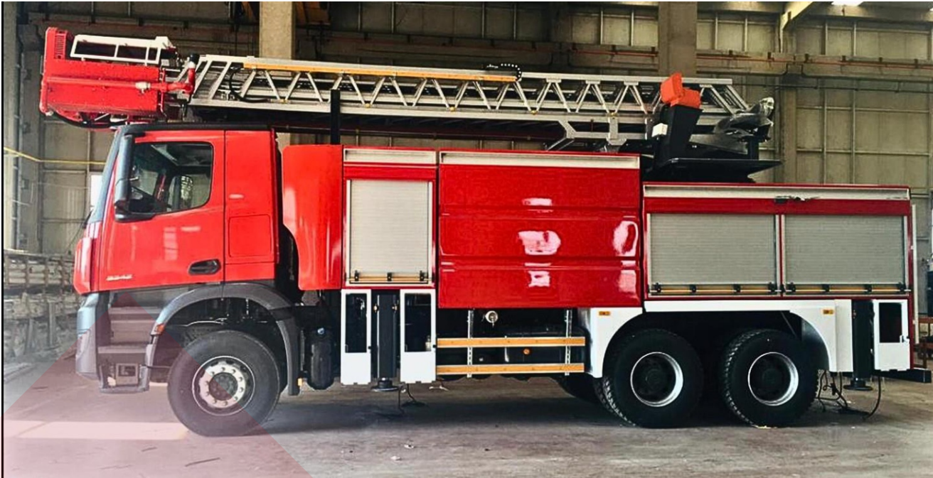
Mercedes Benz Arocs 6x4 Truck; superstructure 28 meters ladder fire extinguishing truck with 4 tons of water + 2 tons of foam tank capacity with folding type basket
